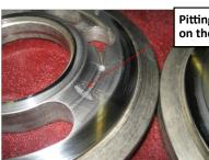
Pitting on this plate was due to dieseling on the pump valve plate
